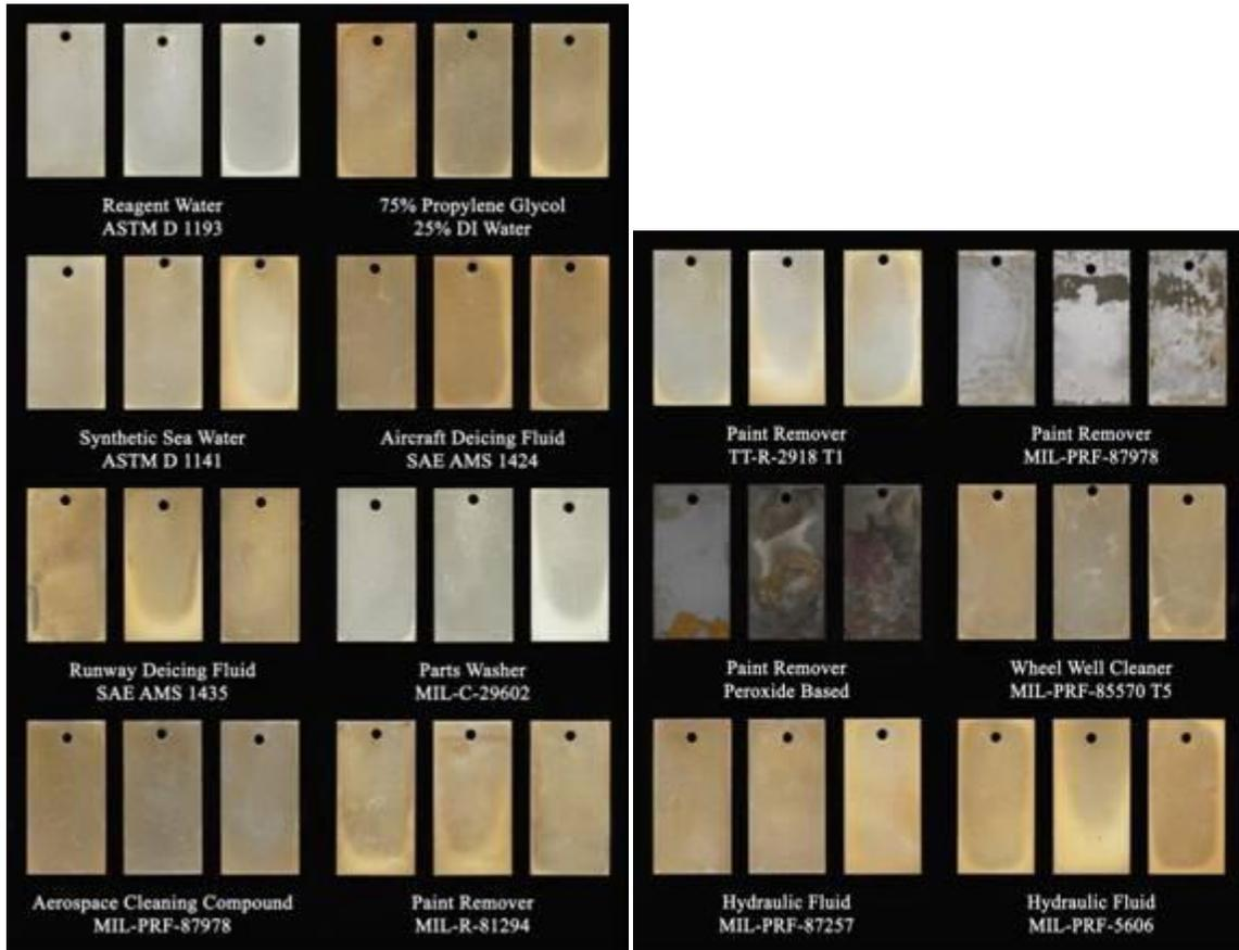
Figure 11. Cd-Plated Panels after Fluid Immersion
