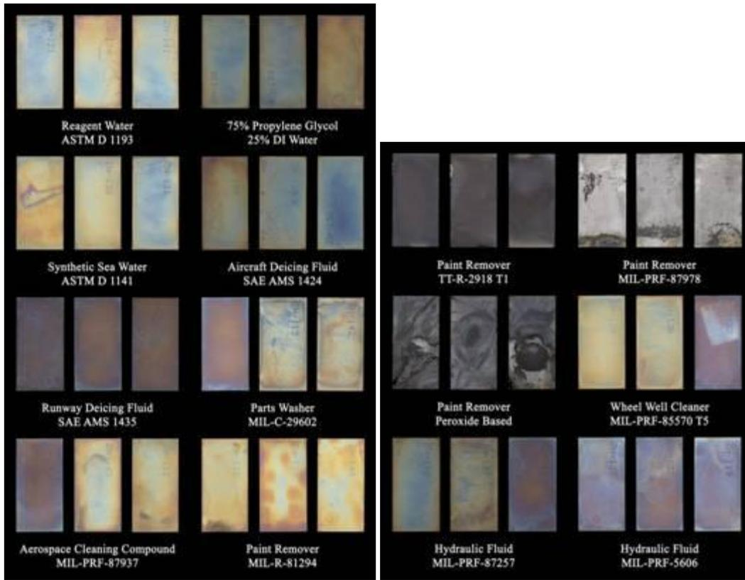
Figure 13. LHE Zn-Ni Panels after Immersion
