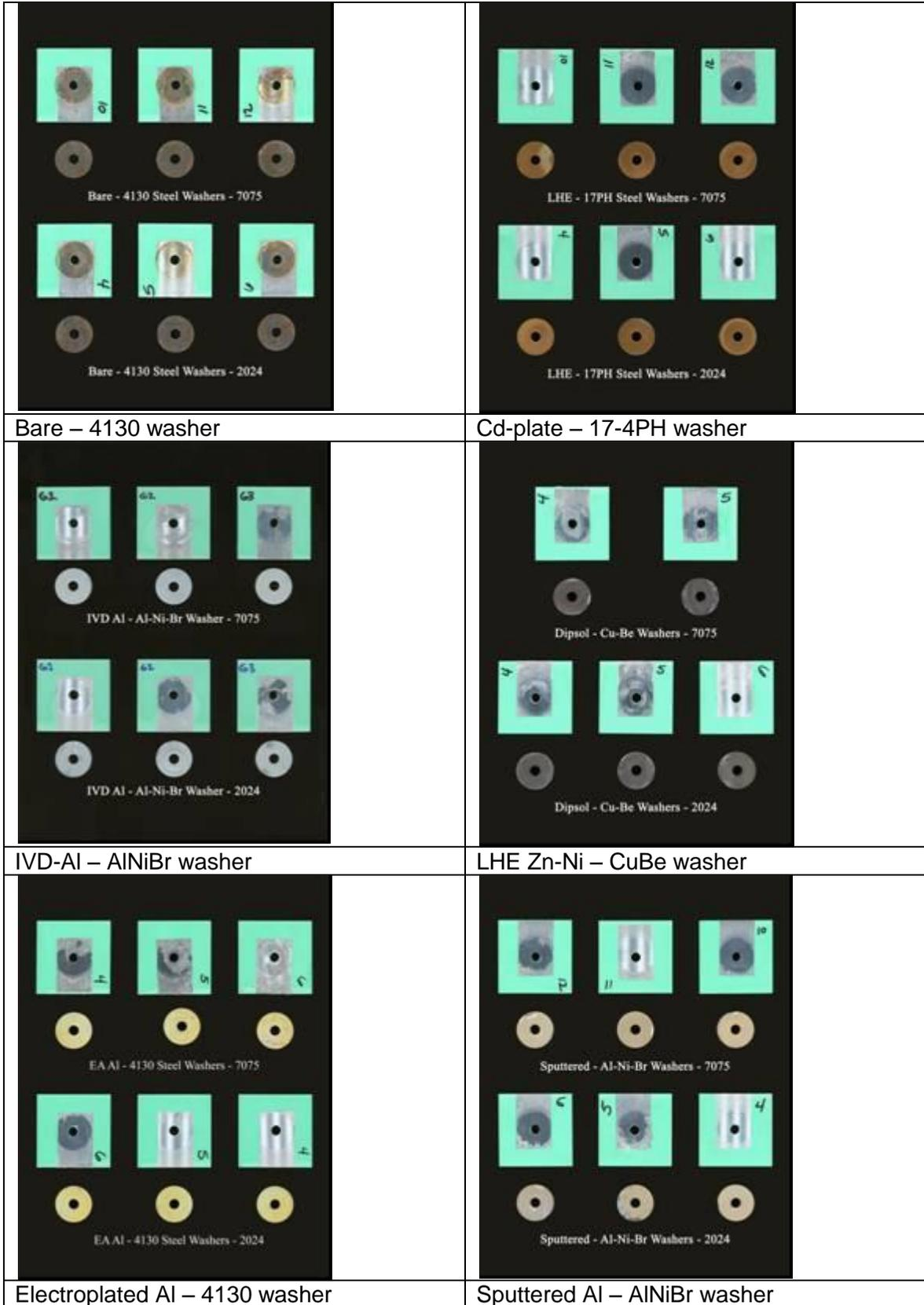
Figure 9. Representative Photos of Cyclic Corrosion-Exposed Fixtures
