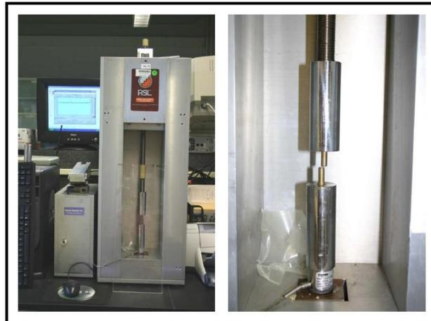
**Figure 39. Hydrogen Embrittlement Test Equipment**
