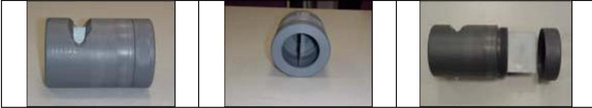
**Figure 1. Fixture for Throwing Power and Alloy Composition Test**
