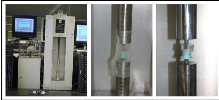
Figure 40. Hydrogen Re-Embrittlement Test Equipment
