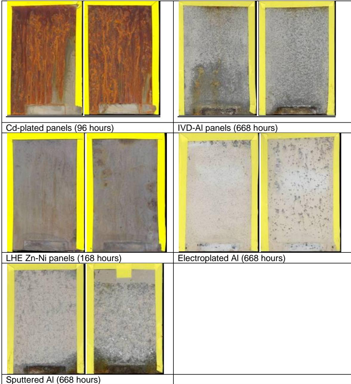
**Figure 18. Representative Photos of SO<sub>2</sub> Salt Fog-Exposed Panels**
